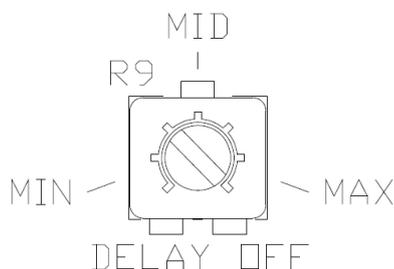
The DEL configuration switch activates the Delay-Off drying cycle timer on the DS-8C. The timer allows the DS-8C to continue to operate and dry the heated surface through evaporation once precipitation has stopped. The drying cycle reduces the chance of moisture left behind refreezing into ice. This timer is restarted by each sensor trigger. Therefore, the DS-8C will continue to operate as long as it is triggered, then for the Delay-Off period once the trigger clears.
