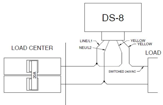
240VAC In, 240VAC Load, Heat Cable or Similar (Strap DS-8 for 240VAC Power)
